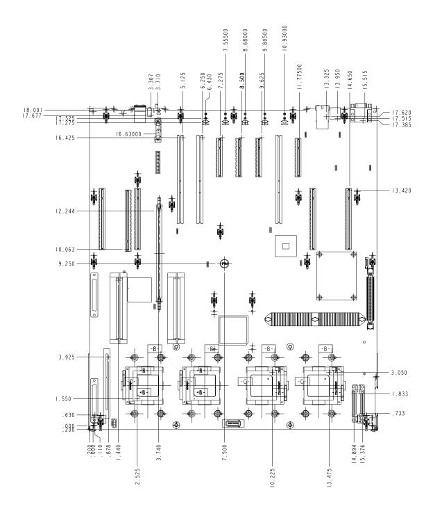
Figure 20. Mainboard Pin 1 Location Drawing
